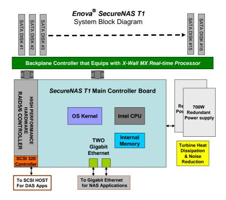
Please reference above *Enova Technology SecureNAS T1* hardware architecture for which *X-Wall MX* sits at the backplane of the high performance hardware RAID 5 and/or RAID 6 storage sub-system and the keys that operate each individually connected SATA disk drive are securely delivered via the Gigabit LAN port through a remote Key Server. Each one of the connected SATA disk drive is controlled by an *X-Wall MX* real-time cryptographic processor, ensuring absolute security over all written data.
